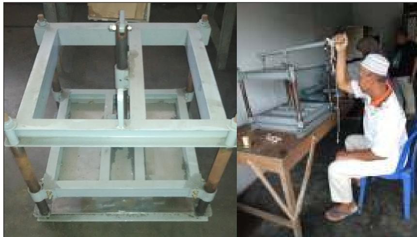
Figure 9. The prototype of pressing machine
